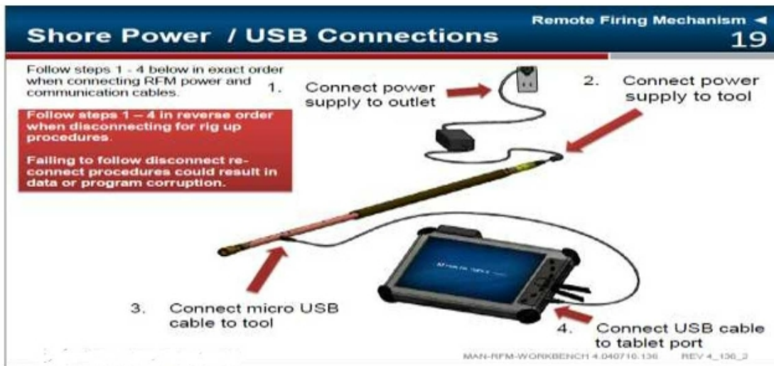
Fig. 8. Set-up of the Remote Firing Mechanism
