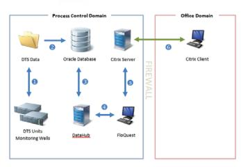
the date range and fiber ID to fetch the data via DataHub (4). A Citrix server located in the PCD provides a connection path between FloQuest (5) and users with Citrix clients (6) in the office domain.
