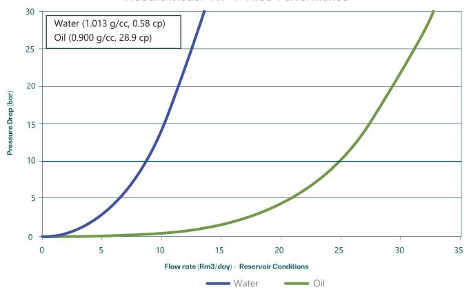
Pressure drop versus flow rate for water and oil is plotted for visualisation of the mobility control imposed by the FloSure AICD. It illustrates flow rate through the valve increasing with 28cp oil compare to water. The mobility ratio between water and heavy is 2.5 times. This implies that water travels faster at similar pressure gradient compare to oil and lead to reduction in water flow at similar pressure drop.
