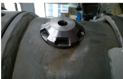
Bypass Valve assembled within ICD housing
