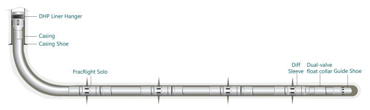
FracRight Diff Sleeve System for Cemented Applications
