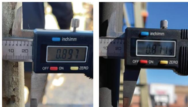
Figure 1 OD measurements taken before and after treatment
