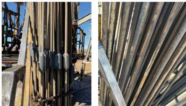
Figure 2 Operator side Pre (left) NORM 237 µR/hr. Post (right) NORM 29-62 µR/hr: after time to dry
