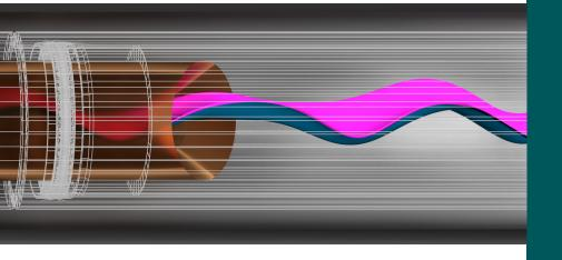
As produced fluids travel through the tool, infinitely variable ports are used to briefly manipulate the flow regime with precision
