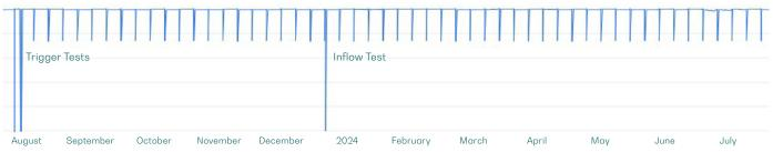
Snap shot of well data, showing trigger testing after install, mid year inflow test and weekly vitality pulses
