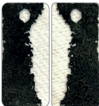
P-110 Alloy in inhibited 15% HCl 149°C (300°F) Acid blend after 6 hours
