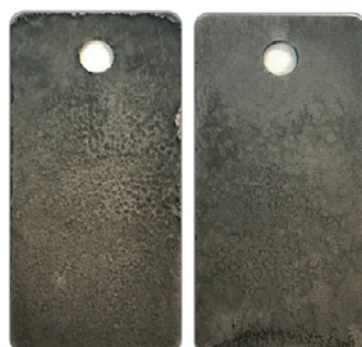
P-110 Alloy in ScaleFix CSD 149°C (300°F) after 6 hours
