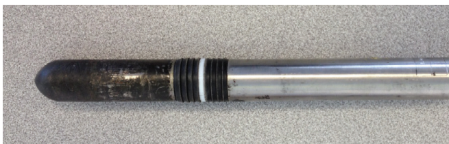
Damaged Gas Lift Valve
