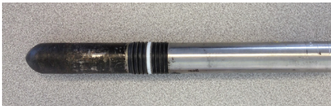
Damaged Gas Lift Valve
